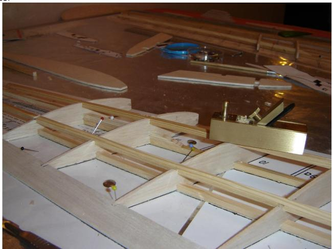
Similarly, next step will be planing the bottom surface of the lower main spars of the wing tips. The lower front spar doesn't need planing or just slightly, but the lower rear spar does.
